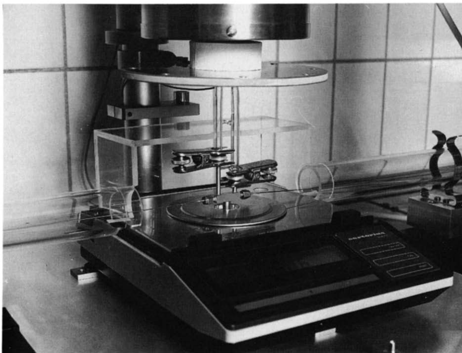
Fig. 2. Tubular reactor-thermobalance, central part of the apparatus.
